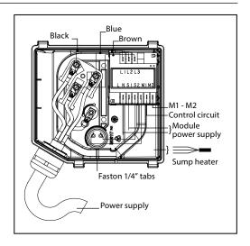
The motor protection module comes preinstalled within the terminal box. Phase sequence protection connections and thermistor connections are pre-wired. The module must be connected to a power supply of the appropriate voltage. The module terminals are 0.25" size Faston type.
