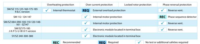
Compressor models SM/SZ084 - 090 - 100 - 110 - 112 - 120 - 124 - 147 - 148 - 161 have been provided with an internal overload motor protection to prevent against excessive current and temperature caused by overloading, low refrigerant flow phase loss or incorrect motor rotation. The cutout current is the MCC value listed in section "Three phase electrical characteristics".
